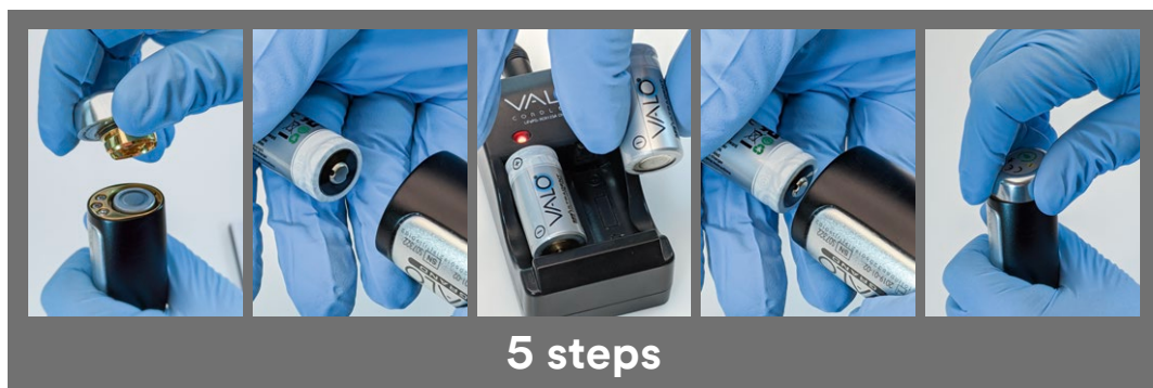
Fig. 7: Battery recharging steps with VALO® Grand LED Curing Light. Source: Ultradent VALO® Grand LED Curing Light Instructions for use no. 1003883.7 080318
