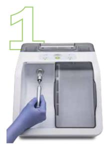
Load a handpiece into chamber one. Slide the window over and press start.
