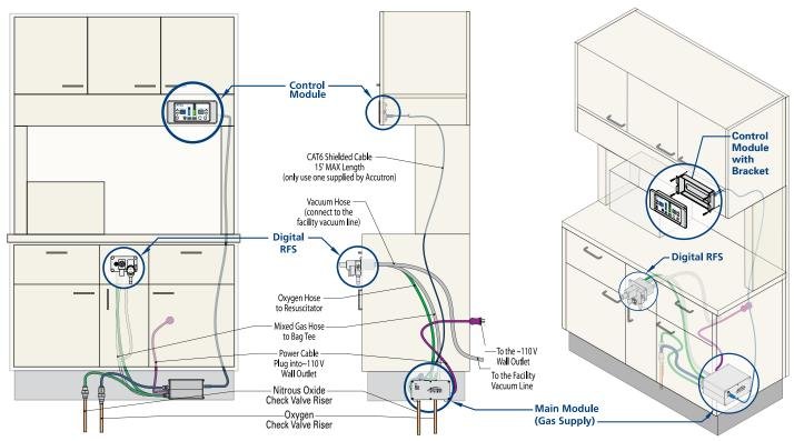
In-cabinet illustrations are specific to 56800 Digital Ultra™ Flushmount with RFS Vacuum Controller.
