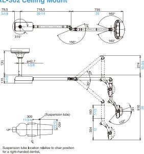
\*Select suspension tube length based upon ceiling height
