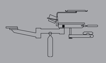
The very popular beneath counter mount is anchored by a half-inch steel plate that can be integrated into your custom made rear cabinet, or as part of a Modular & Custom Cabinetry rear cabinet (PFR8144), which includes the steel plate preinstalled.
