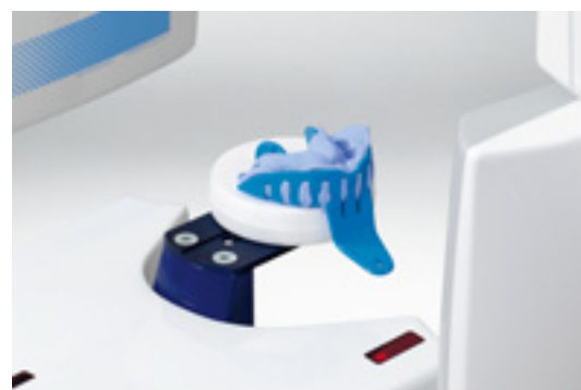
Scanning an impression to a digital model
