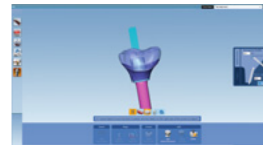
Emergence profile design for a one-piece hybrid abutment
